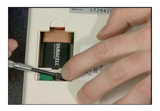
Using a flat head screwdriver gently pry one side up and the other side to remove the chip.
